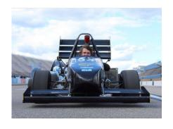
CB6 is our most refined car to date, marking another milestone for CU Racing. This vehicle passed all technical inspections and completed every dynamic event at the 2025 FSAE Michigan IC competition, delivering competitive times across acceleration, skidpad, autocross, and endurance. Building on CB5's innovations, CB6 featured an optimized aerodynamics package, refined suspension geometry, and further weight reduction, all contributing to its strong overall results.
