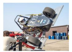
CB5 competed in the 2024 FSAE IC Michigan competition. CB5 was our first ever vehicle with an aerodynamics package and a differential. This ambitious design cycle has the most YoY changes to date. Other key changes to this platform include moving away from the direct linkage front suspension showcased in CB4, as well as a thirty percent power increase as a result of a new and improved intake system.
